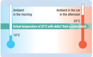
delta T fluid elements maintain the inner temperature of the transport box within the allowed range. Hereby, the conditions of the ambient temperature around the
